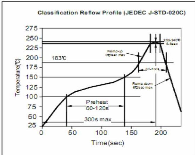
**Soldering Profile for Lead Free Soldering**
